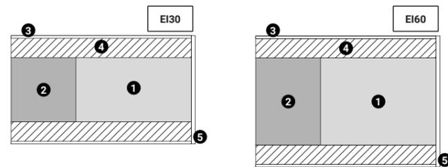
1. Bastidor perimetral 800kg/m<sup>3</sup> 100x30mm (EI30) / 100x40mm (EI60)
